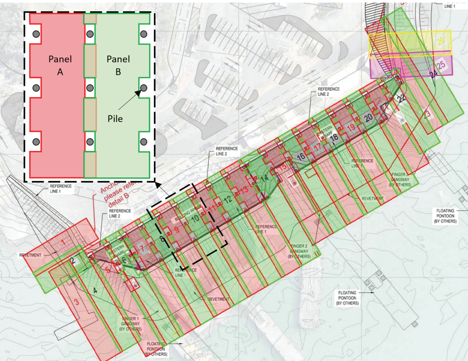
Layout plan of revetment with fabricated Mirafi® PET2000/100 kN/m customized panels
